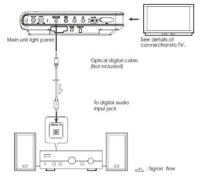
Carefully check the player s digital output settings before connecting the player to an amplifier equipped with a digital audio input jack which is not Dolby Digital / DTS / MPEG compatible.
